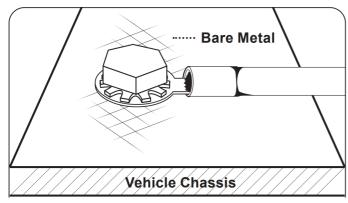
NOTE: Remove any paint below the ring connector for proper grounding.
