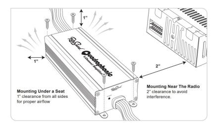
The compact size of the Retro Sound® Quadraphonic amplifier enable sconsiderable installation flexibility. For example, the amplifier may be placed behind the dash or under the seats. It is best to mount the amplifier in a location that allows air to freely circulate around it and allows access to the end panel controls for adjustments. Although both thermal and overload protection are built in, if the amplifier overheats it will reduce its power output to maintain operation.
