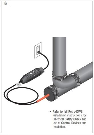
6. Plug in heater and Test/Reset GFCI located in cord set (GFC models).
