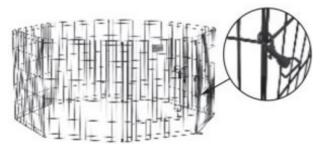
4. For added safety, install a Ground Anchor at the intersection of each panel.
