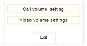
**Call volume setting:** Select the Prompt Volume Setting option, click OK button to enter the setting mode, set the volume up or down by pressing the Forwardand () and Backward() buttons. Click Exit to return after selecting.
