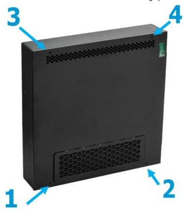
**Step** 2 – Remove screws "1 and 2" using a PH1 Phillips head screwdriver.
