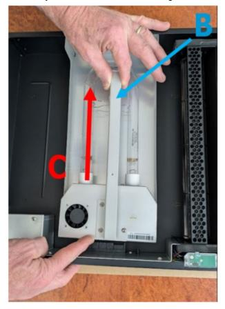
**Step** 5 – Gently clean the optic with a lint-free cloth. Ensure optic is completely dry before re-insertion.
