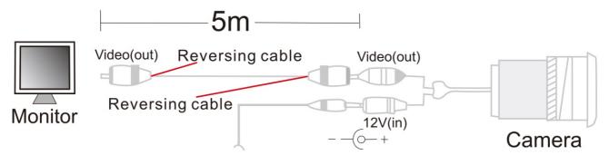
Yellow socket is connected to video Power socket is connected to DC 12V
