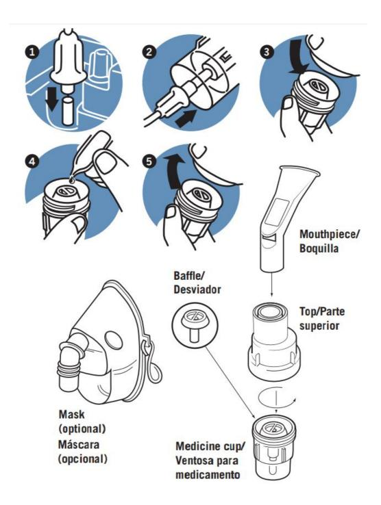
The SideStream is a compressor-driven nebulizer designed to convert liquid medication into aerosol for inhalation by the patient.
