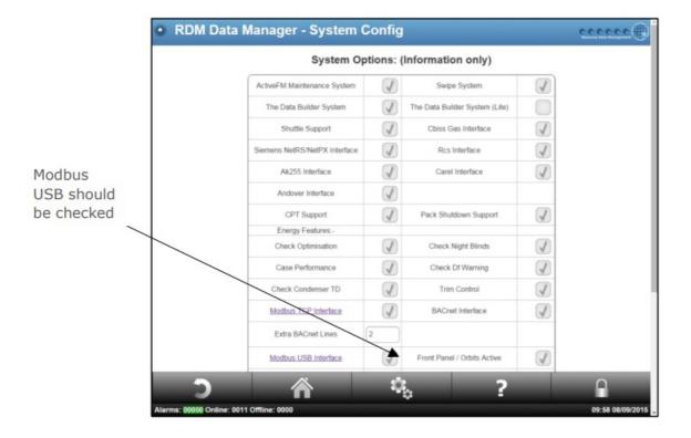
When activated, it will open a number of useable 'templates' for devices to communicate with the DMTouch. Currently the following Modbus® devices are supported:
