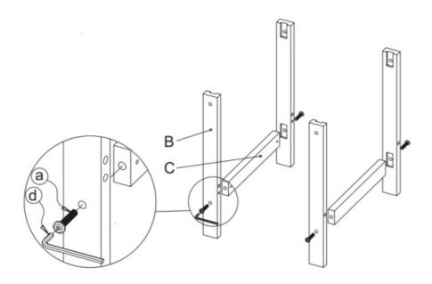
**Step 2:** Take out D and install it on B with c and b (as shown in the figure below).
