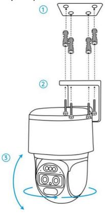
Note: Use the drywall anchors included in the package if needed.
