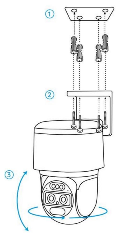
$\textbf{Note:} \ \textbf{Use the drywall anchors included in the package if needed}.$
