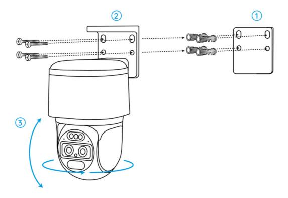
**Note:** If you install the camera on a pretty hard surface such as drywall, use the drywall anchors included in the package.
