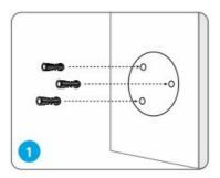
Install the mount base with the mounting screws included in the package.
