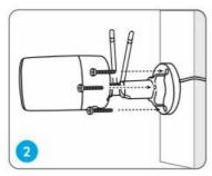
• To get the best field of view, loosen the adjustment knob on security mount and turn the camera.
