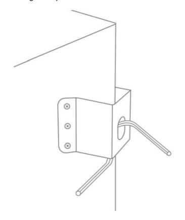
Then, screw the camera to the bracket according to the holes and adjust the cameraangle for the best coverage.
