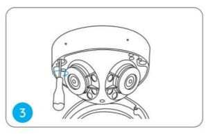
Adjust the camera's viewing angle as needed.
