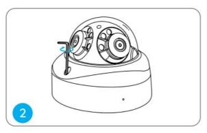
Screw the camera base to the ceiling.
