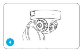
Attach the dome cover to the camera base by tightening the screws.
