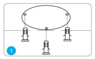
Screw the dome cover off the camera base with the hex key.
