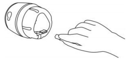
2. Insert the battery into the camera and tighten the back cover.
