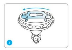
Rotate to separate parts from the bracket.
