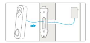
**NOTE:** Reolink Video Doorbell PoE&Wi-Fi can also be powered by the existing doorbell wiring system. In such case, you are required to first bypass the existing mechanical chime with the jumper cable to get
