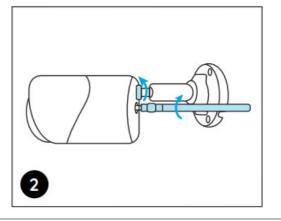
Drill holes in accordance with a mounting hole templat e and screw the security mount into the wall. If you are mounting the camera on any hard surface, i nsert plastic anchors into the holes first.
