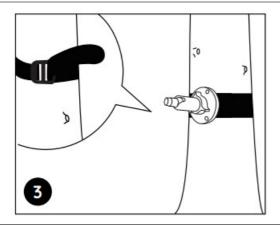
Lose the adjusting knob on the mount and adjust the c amera to the proper direction.
