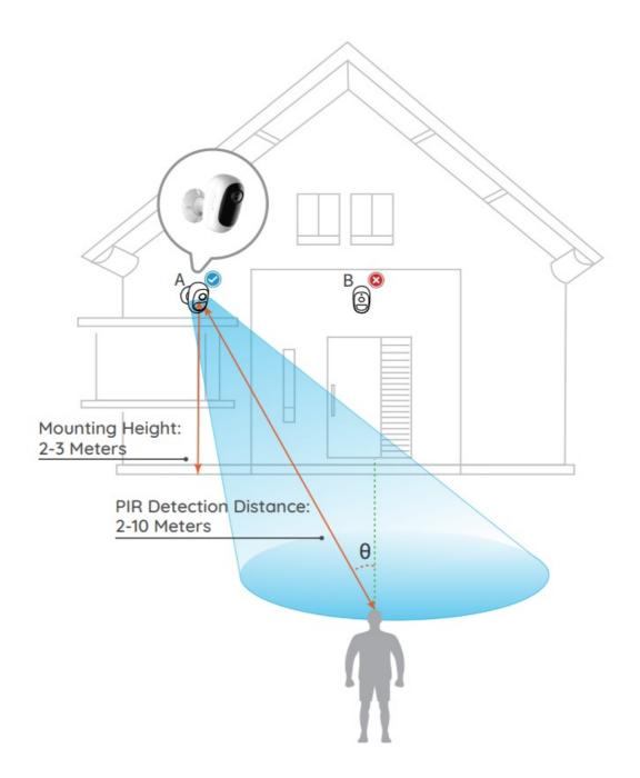
**NOTE**: If a moving object approaches the PIR sensor vertically, the camera may fail to detect motion.
