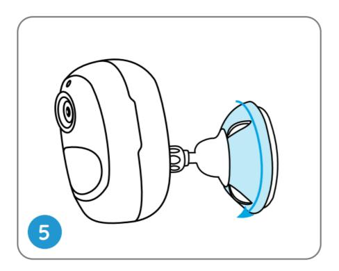
**NOTE**: To adjust the camera angle later, please loosen the mount by turning the upper part anticlockwise.
