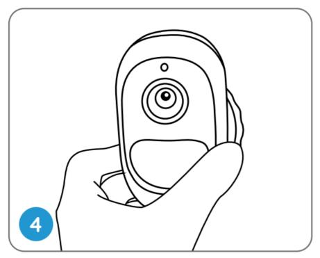
5. Secure the camera by turning the part on the mount identified in the chart clockwise.
