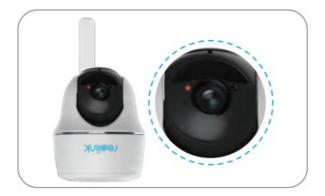
A blue LED will flash for a few seconds and then go solid before going out. You will hear a voice prompt "Network connection succeeded", which means the camera has been successfully connected to the network.
