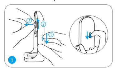
Install the bracket to the ceiling. Align the camera with the bracket and turn the camera unit clockwise to lock it in position.
