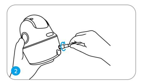
3. Screw the camera to the security mount and adjust to the proper direction.
