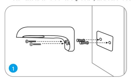
**NOTE:** Use the drywall anchors included in the package if needed.
