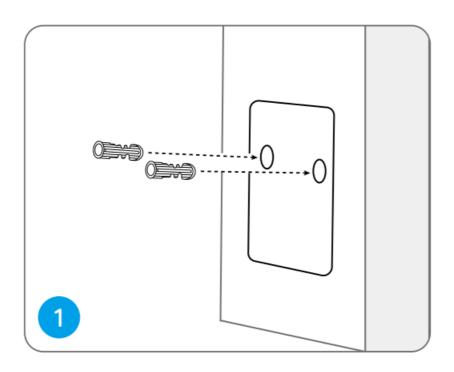
Drill holes in accordance with the mounting hole template.
