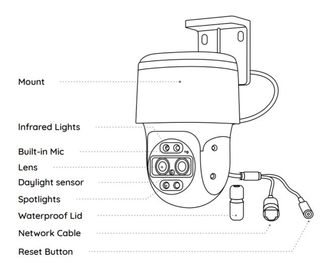
• Press for about 10 seconds to restore the device to factory settings.
