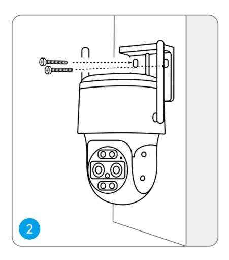
Install the mount base with screws included in the package.
