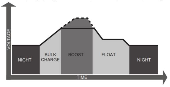
**Bulk Charge:** This algorithm is used for day-to-day charging. It uses 100% of available solar power to recharge the battery and is equivalent to constant current.
