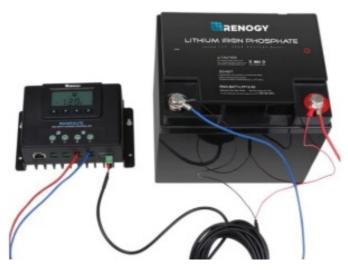
6. Verify successful connection by making sure that the green connector is pressed firmly in the port or by using a multi-meter to read the respective battery terminals on the screws.
