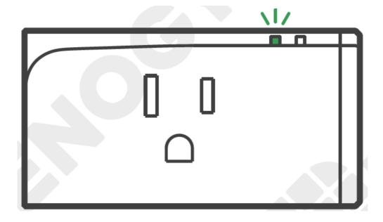
For initial use, Smart Plug (Zigbee) enters the pairing mode upon power on with the LED signal indicator flashing green.
