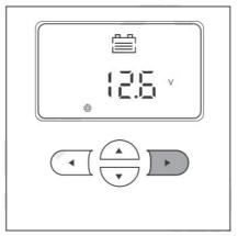
12. Press or value adjust the overdischarge return voltage according to the usage.
