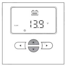
11. Press box to set the overdischarge return voltage.
