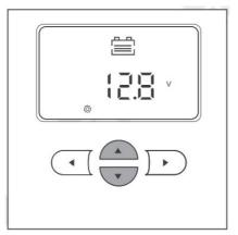
13. Press boto set the overdischarge voltage.
