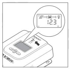
8. Once the Solar Panel Extension Cables are connected to the solar panels, the Solar LED Indicator will light up, and the charge controller enters daytime mode.
