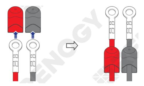
Step 6. Install Battery Terminals
