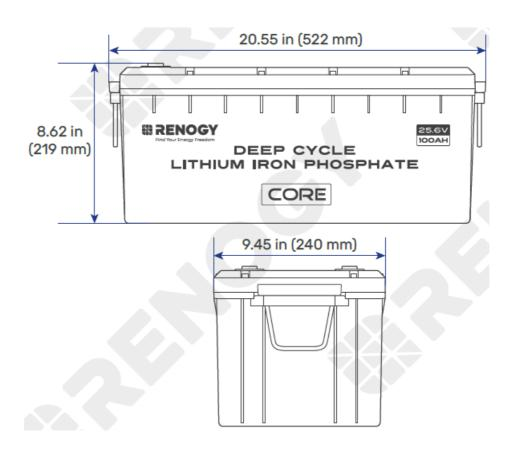
• Dimension tolerance: ±0.2 in (0.5 mm)
