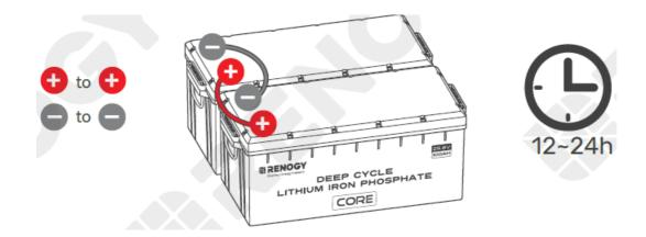
It is recommended to periodically rebalance the battery voltages every six months when connecting multiple batteries as a battery system. Slight voltage differences can occur among batteries over time due to factors like battery chemistry, capacity, temperature, and usage patterns.
