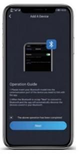
4. When a device is found, select the Bluetooth device, then name the device if you wish. Afterward, press "Next" and then select the type of device you are connecting. In this example, we will select Charge Controller. When successful, the App will confirm the product SKU. If the SKU is correct, click"OK" to start communicating with your Rover 30Amp.
