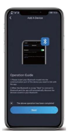
4. When a device is found, select the Bluetooth device, then name the device if you wish. Afterwards, press "Next" and then select the type of device you are connecting. In this example, we will select Charge Controller. When successful, the App will confirm the product SKU. If the SKU is correct, click "OK" to start communicating with your Rover 30Amp.
