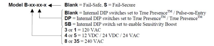
**NOTE:** Models B-3, B-4 and B-8 are fitted with a rear mounted, 11-pin, Amphenol style connector. Models B-1, B-5, and B-35 are fitted with a rear mounted, 10-pin, MS style connector.
