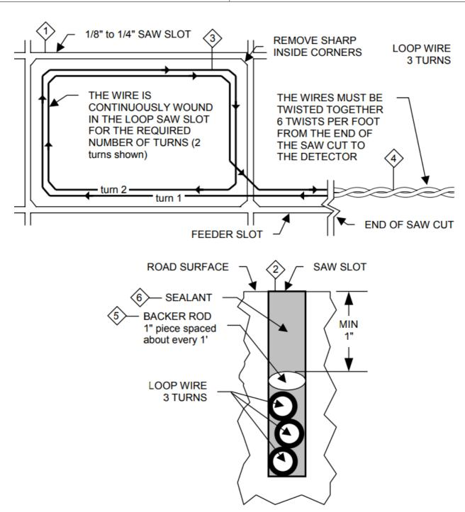
• Recommended Loop Wire: Reno A&E LW-120 for 1/8" slots Reno A&E LW-116-S for 1/4" slots
