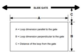
As the length of leg A is increased, distance C must also increase. For reliable detection of small motorcycles, legs A and B should not exceed 6 feet.
