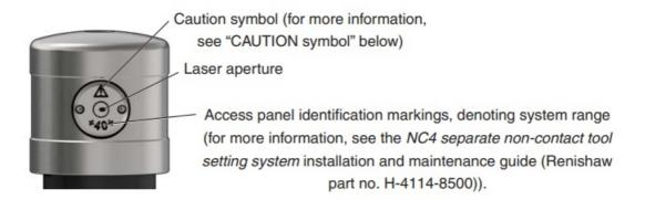
The access panel is to be removed for service purposes only, using the special tool supplied.
