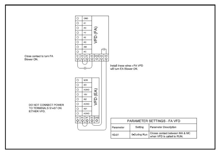
FIGURE 2.2.2 ALTERNATE CONTROL WIRING
