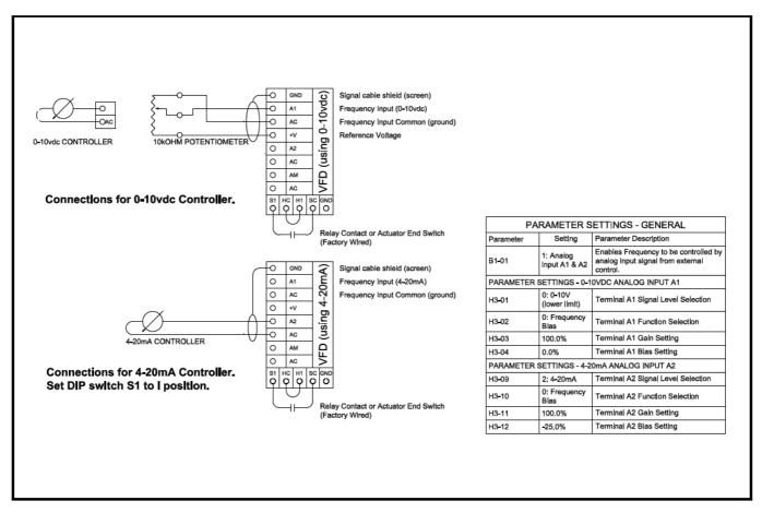
FIGURE 2.2.3 EXAMPLES OF ANALOG INPUT CONNECTIONS
