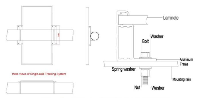
Illustration of single-axis tracking system installation
