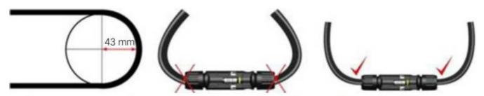
The correct routing and minimum bending radius of cables.
