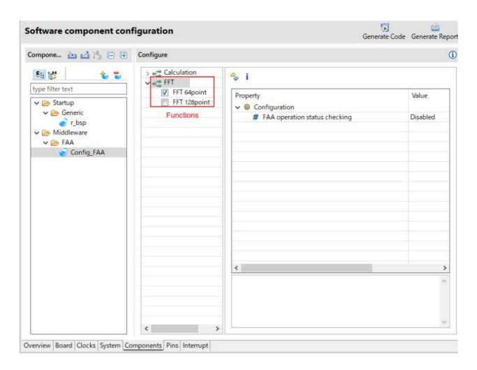
1. Select FFT points to be used in the Functions of smart configurator.
