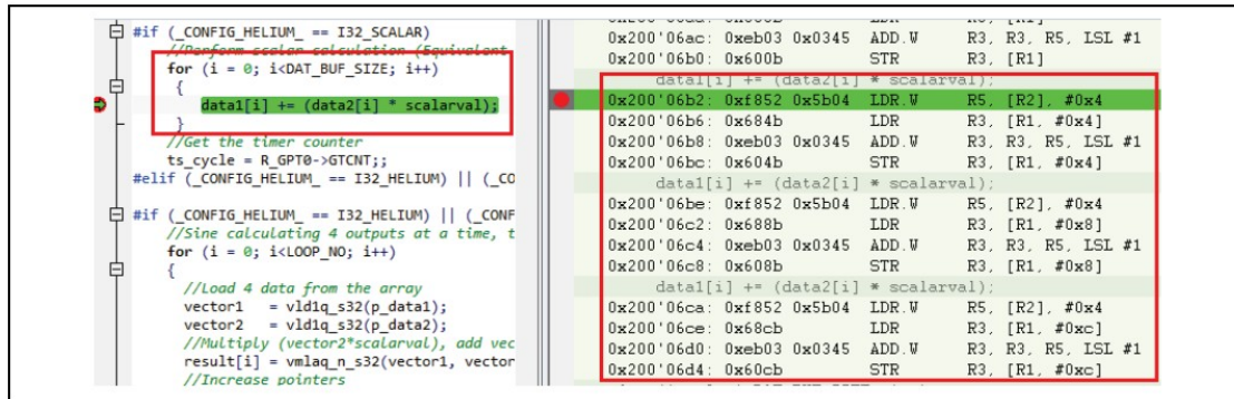
Figure 16. Example of Scalar Code Equivalent of VMLA and Disassembly Code
