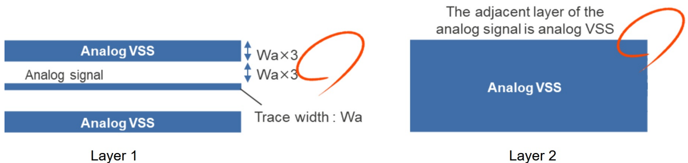
Figure 17, Recommended design image: Example of shielded trace Top View)
