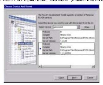
• In the "Choose Device And Kernel" dialog, select the EDK target device from the drop down list: "H8S/2282F"
