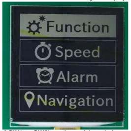
m. Pressing the user switch (one of SW1 to SW2) on the mainboard changes the image on the MIP-LCD. The following is the image after pressing SW1.
