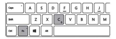
Press FN+C at the same time to enable pairing mode.
