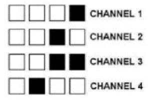
Press button 3 repeatedly until the channels lights indicate one of the output channels you wish to program. Select a channel that you wish to operate with a remote control i.e. not a channel that you wish to operate with a wireless detector.
