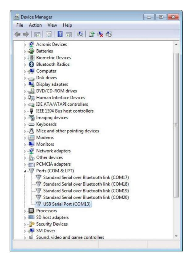
**Note:** The USB Light will on the ZUSB communications module only illuminate if the virtual COM port driver is properly installed. If the device remains undetected, try disconnecting and reconnecting the power and USB cables.
