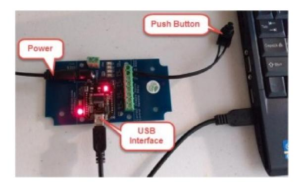
3. Run N-Button Pro/Lite software. Click Device Manager -> New to add USB push notification board **Manufacturer** -> National Control Devices
