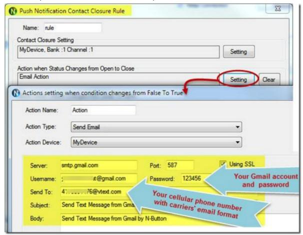
3. After finishing all the above settings, all recipients will receive an email once the contact closure input on the board changes state. To test, close the contact input on the push notification board and check your email **Note**: If you use Gmail, you need to turn on "Allow less secure apps" on your Gmail Account —> Sign-in security panel, shown as below.
