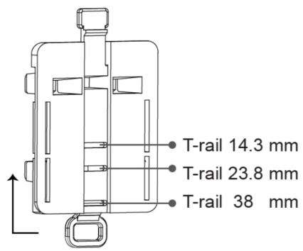
Slide the AP into the T-rail mount which works similar to the wall mount.
