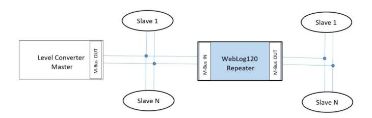
• The M-Bus line of the existing master or level converter is connected to the terminals marked M-Bus Repeater.
