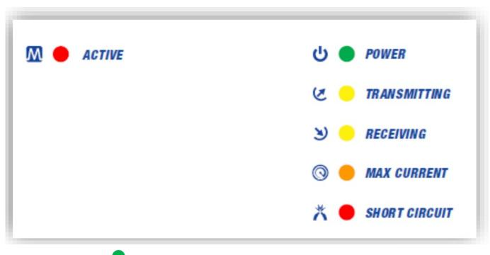
The M-Bus output voltage is switched on.
