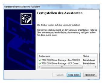
Now you can connect the PC. The USB driver for the PW250 is installed automatically and generates a new, virtual COM port. The new COM port number of the USB serial port is displayed after the installation is finished (here: COM29). You can look up this number at any time in the Device Manager under ports (USB Serial Port) and – if desired – change it in the advanced settings of the driver. Please select the appropriate comport number in your M-Bus software.
