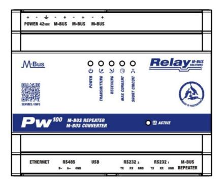
All terminals are pluggable and thus make wiring and replacement of the PW100 easier in the event of a fault. **Attention:** Please make sure to put the clamps back in the correct place after removing them. Incorrectly positioned terminals can lead to defects.
