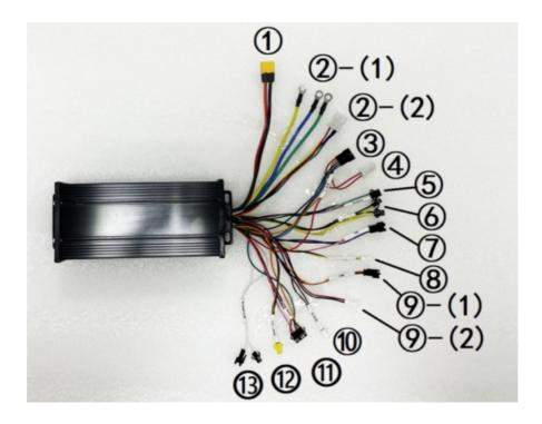
1. Power Supply Plug (Power input to Controller): Yellow XT60 Male Plug
