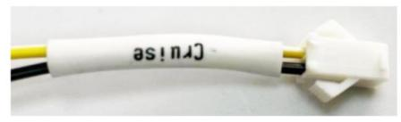
(2). With the jumper plug connected: The cruise function is activated (if you keep the throttle at definitely fixed
