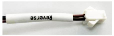
(2). With jumper plug connected: Rotate backward
