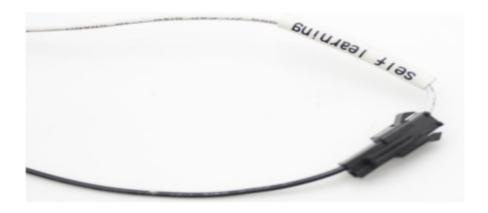
(2). Disconnected: Deactive self-learning (After self-learning, please disconnect plugs) Before you connect the motor with the controller, please be sure these two plugs are disconnected
