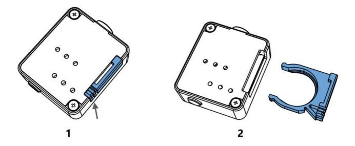
Turn over the light meter and pinch the lower corner of the battery holder with your fingers (shown by arrow in Fig. 1) to remove the battery holder; Then, place the battery (CR1632), positive side up, into the battery holder (Fig. 3) and fit it into the light meter (Fig. 4).
