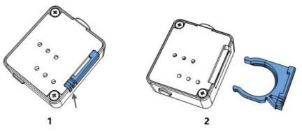
Hold the light meter face down, and pinch the lower corner of the battery holder with your fingers (shown in Fig. 1) to remove the battery holder. Next, place the CR1632 battery into the holder positive side up (Fig. 3). Finally, slide the battery holder back into the battery slot (Fig. 4).
