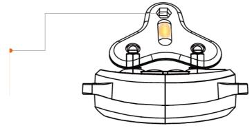
**Note:** The hexagon hole on the Test Bulb Tool can be used to fasten or unfasten the Probes to the Contact Points.
