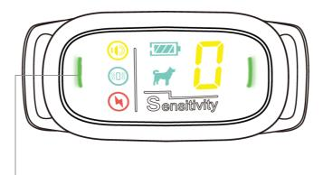
Sett he Bark Control Collar to Test Mode, the display will show digit 0.After that, imitate a dog bark towards the sensor Mic located at the back
