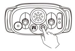
1. Power on the product by pressing and holding the Power Button for 2 seconds
