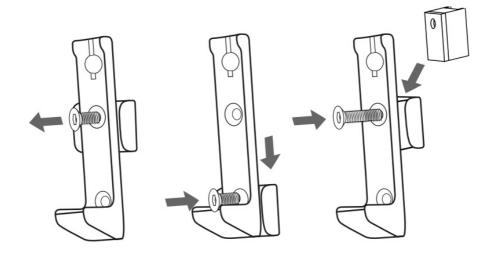
\*NOTE: Do not over-tighten the screw. Should be snug, with no more than 1Nm torque.
