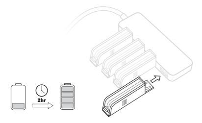
STEP 1: Remove Light Modules from the charger and insert them into Multi Mount. You should hear a magnetic click.
