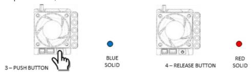
Pull the throttle trigger to the full throttle position, the blue led blinks three times and the motor beeps once, the full throttle position is saved.
